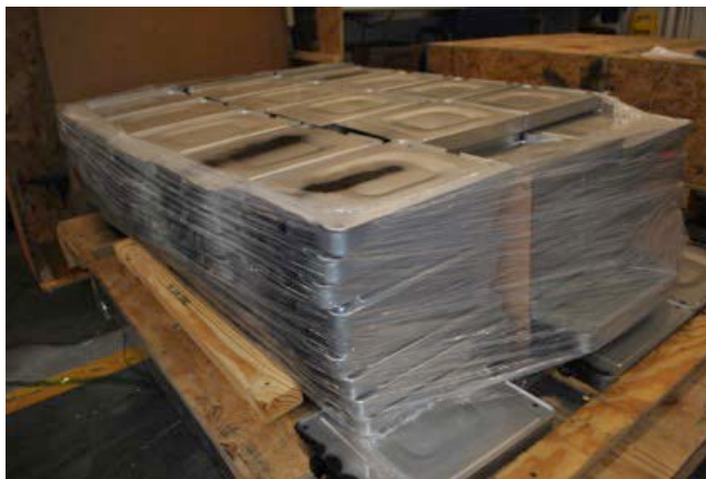
Second life lithium ion batteries donated by 4R energy (owned by Nissan and Sumitomo corp.). We received 1080 modules (approximately 320 kWh) of second used lithium ion battery modules. These modules come from 20 Nissan Leaf electric vehicles.
