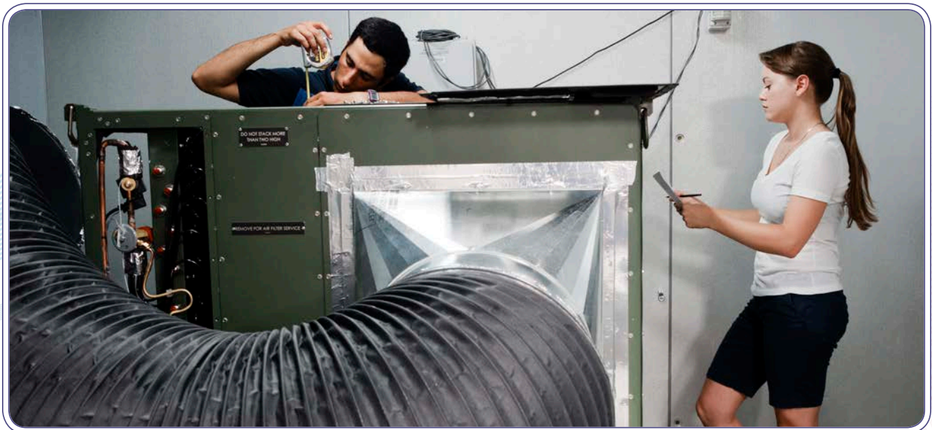
WCEC Student researchers, Cyrus Ghandi and Kaitlyn Thatcher finish instrumenting a rooftop unit for testing in WCEC's environment chamber. Photo: Paul Fortunato
