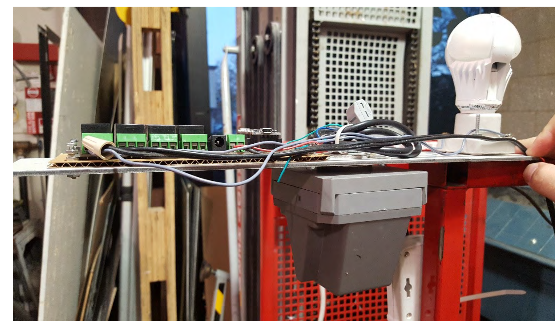
Figure 3a. Microwave Technology — Test Sensor 4 connected to mounting bracket with a trigger-able lighting load.
