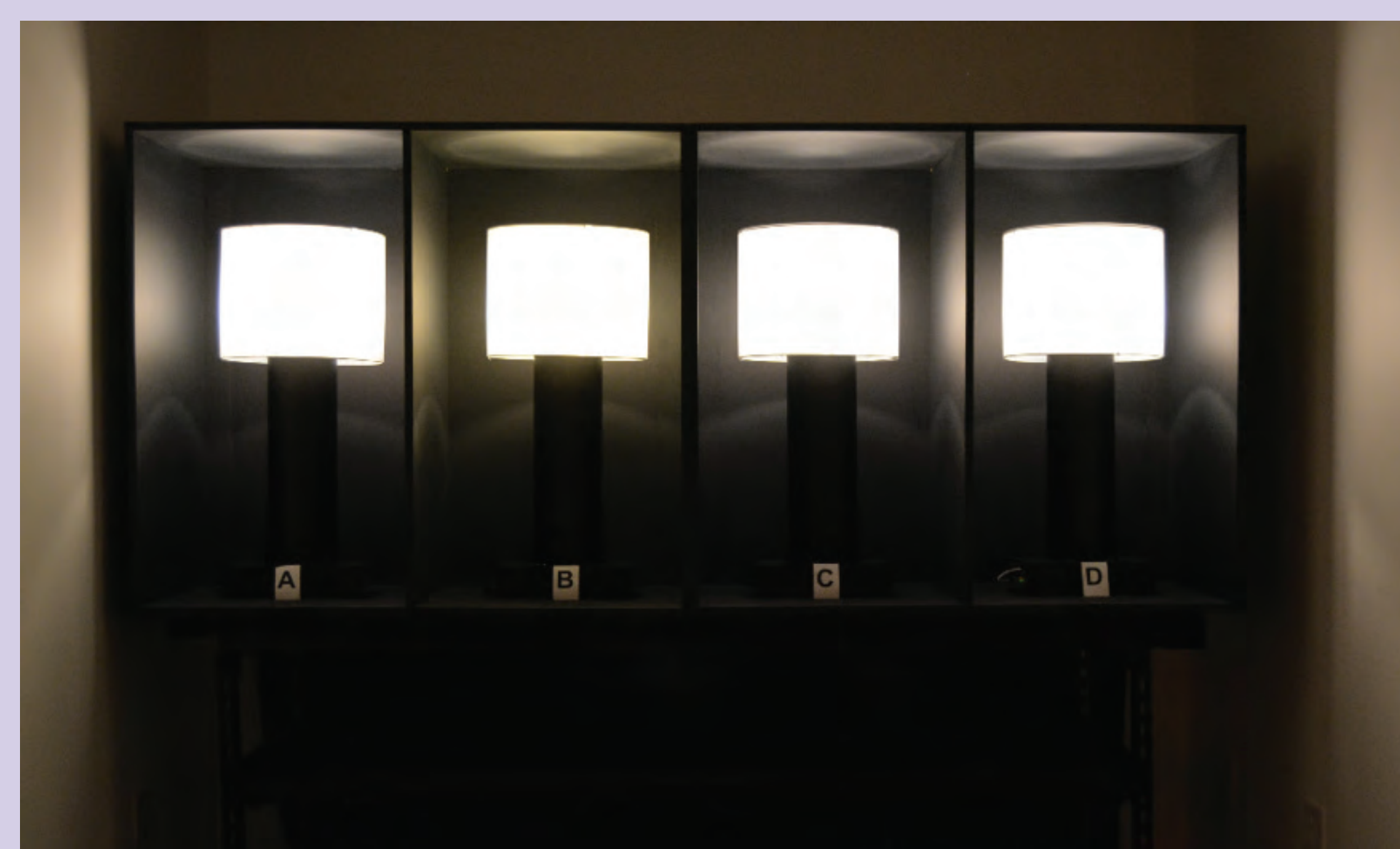
Figure 1a. Color binning test setup at CLTC laboratory
