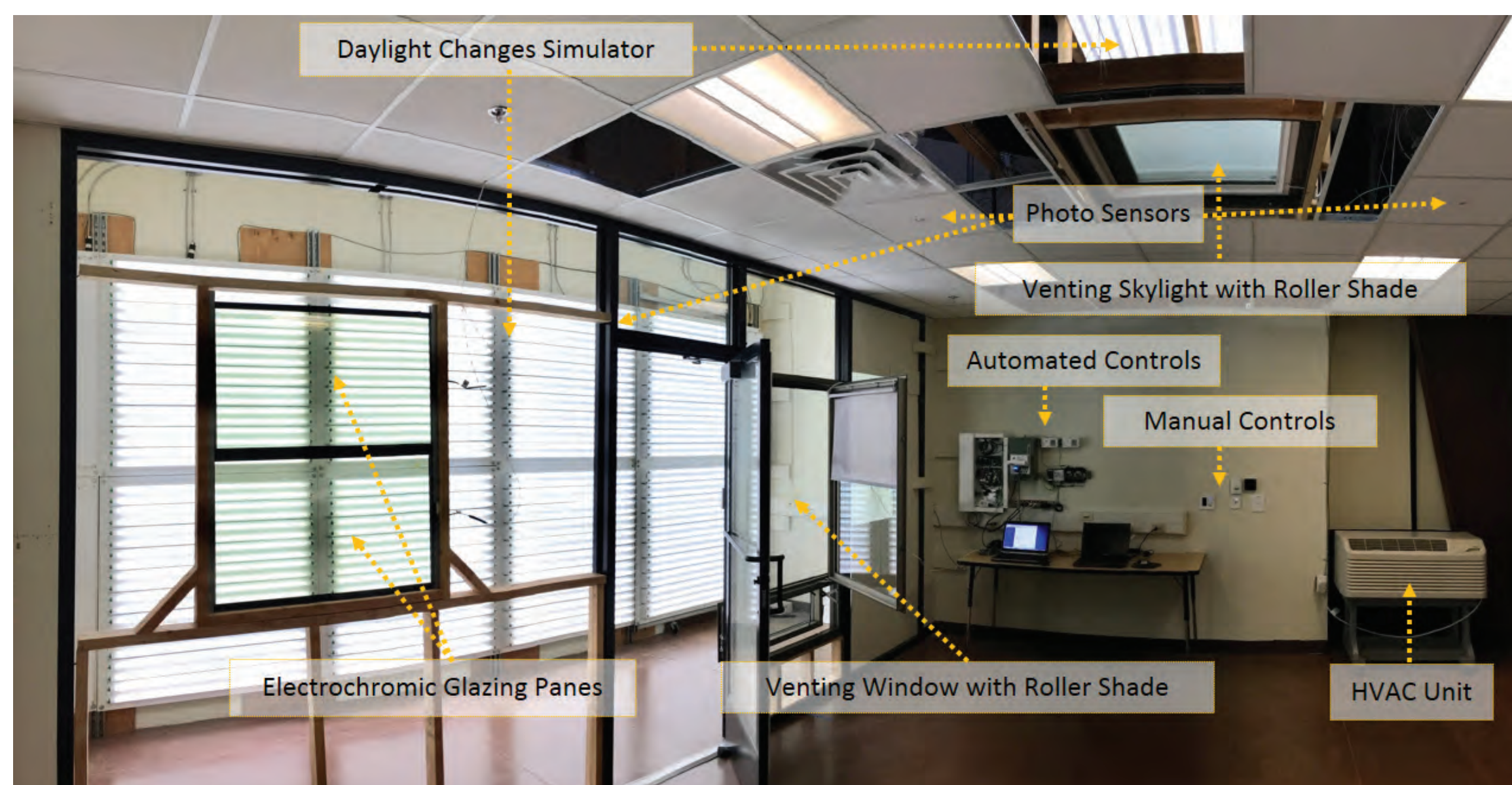
Figure 2. Integrated Building Controls Laboratory at CLTC
