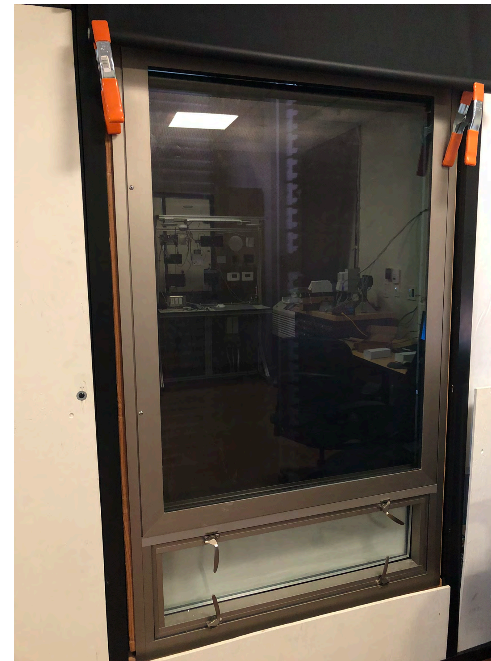
Figure 6. Venting window with adjustable rolling solar film
