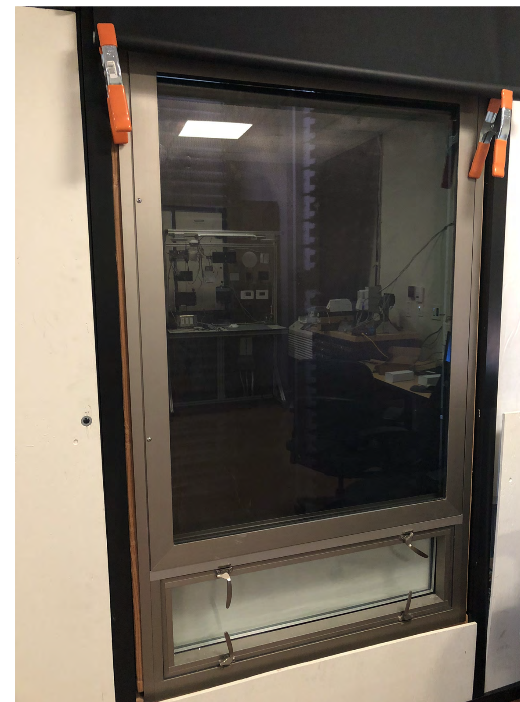
Figure 6. Venting window with adjustable rolling solar film
