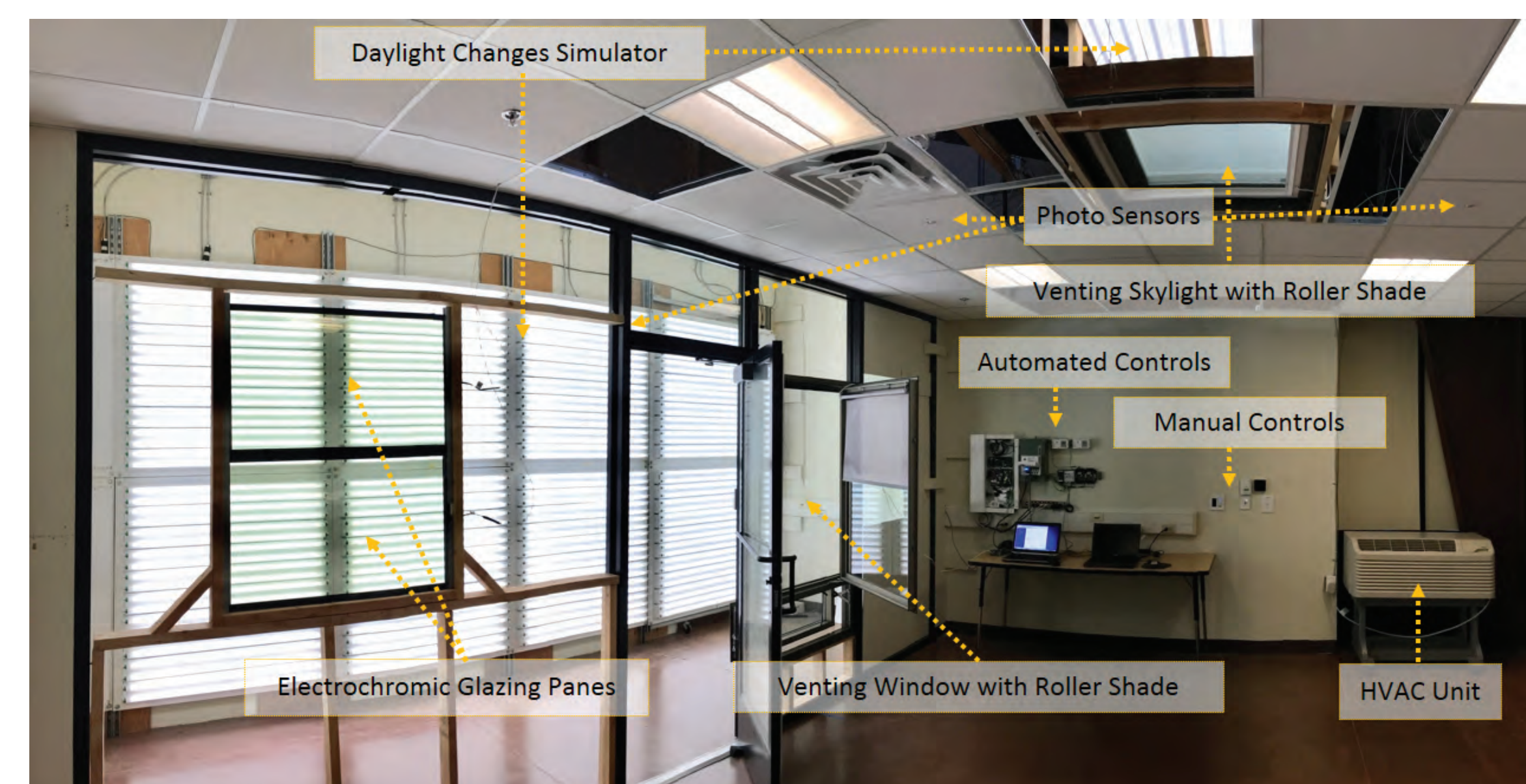
Figure 2. Integrated Building Controls Laboratory at CLTC
