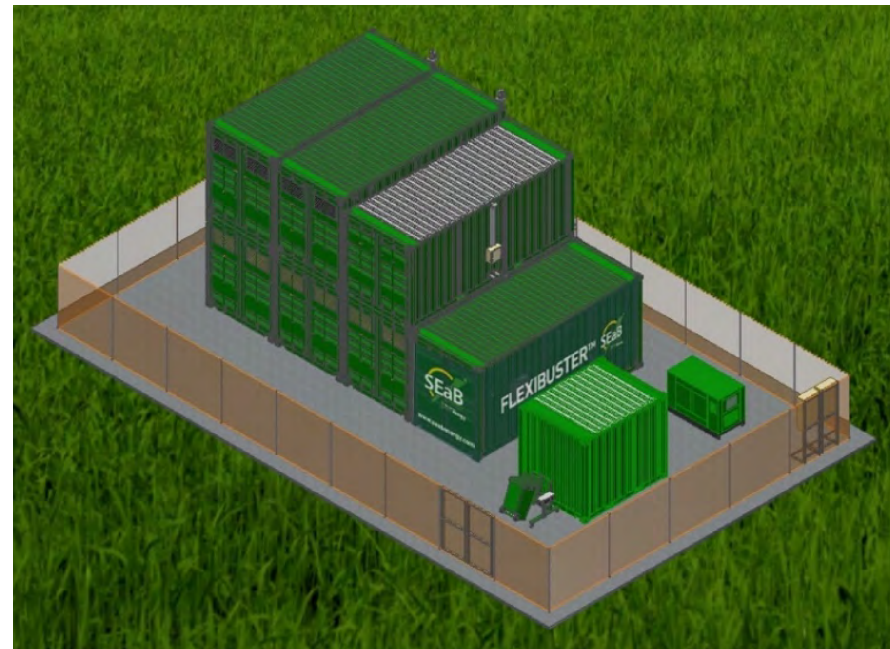
Figure 2a. Small-scale containerized AD unit. This image shows 5 digesters, 1 gasholder, a mouth unit, command unit, and a CHP unit.
