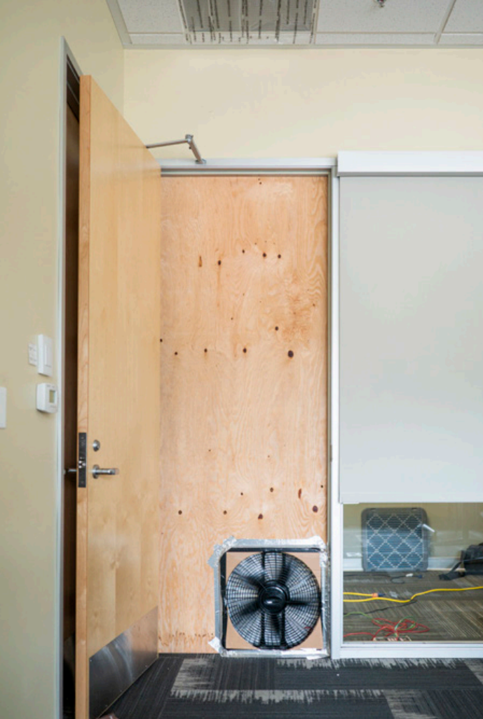
Figure 3 - Flow rate measurement using calibrated blower door
