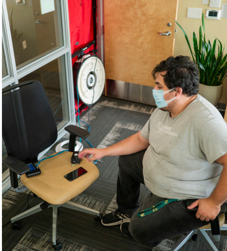
Figure 3 - Flow rate measurement using calibrated blower door
