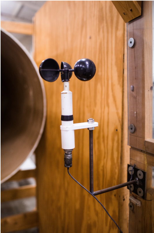
An anemometer (wind-speed meter) at the National Wind Institute at Texas Tech University. PHOTO: DYLAN COLE FOR THE WALL STREET JOURNAL
